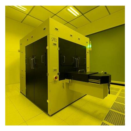
EVG 770 NT enables large-area fabrication of nano-structures for AR waveguides, optics, and biomedical chips.
