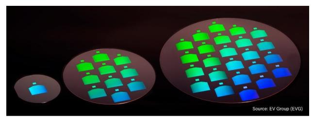
Production scaling enabled by large-area step-and-repeat mastering. Augmented reality (AR) waveguide master courtesy of WaveOptics.
